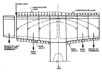
Fig. 4 Segmental Construction Loads
