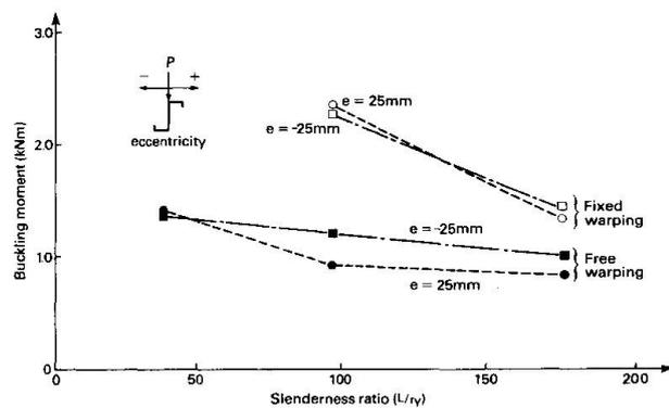
**Fig. 7** Influence of warping restraint on buckling moment
