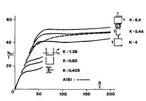
Fig. 11. Effective widths
