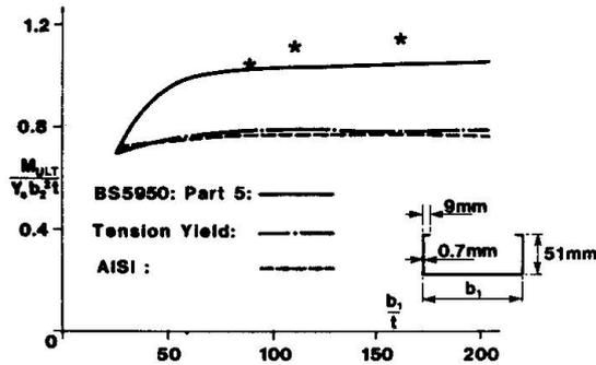
Fig. 13. Failure moments for channels with small lips
