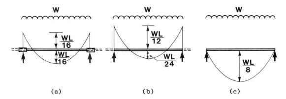
Fig. 3. Bending moment diagrams for purlins
