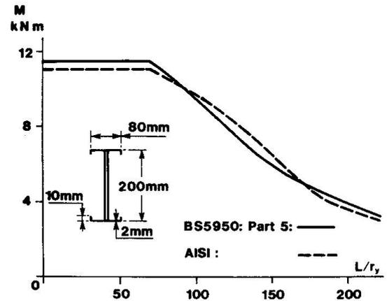
Fig. 14. Lateral buckling capacity of I section beam
