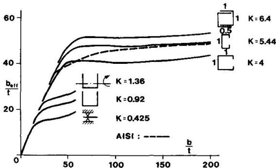
Fig. 11. Effective widths
