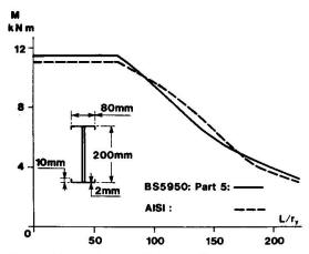
Fig. 14. Lateral buckling capacity of I section beam
