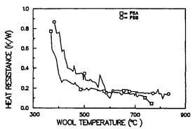
Fig. 9. Heat resistance vs. average temperature
