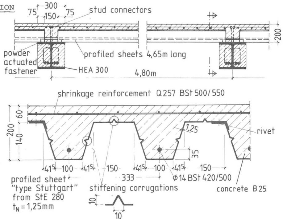
Fig. 8 Sheet-supported reinforced concrete slab in demo-building
