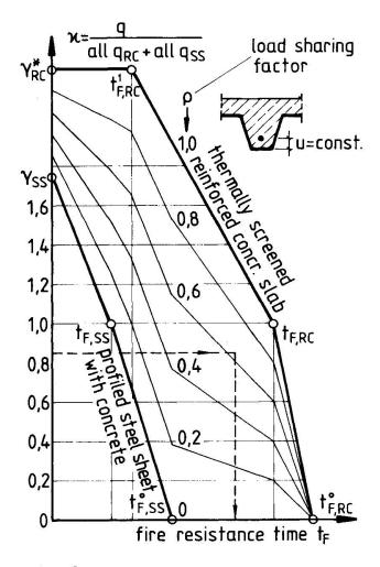
type, nondimensional load bearing capacities (related to the allowable load all  $q_{RC}$  + all  $q_{SS}$ ) versus  $t_F$ . The curves are, according to their load sharing factor (equ. 2), linearly interpolated between the two limiting cases of the sheet-supported RC-slab:
