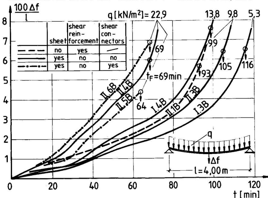
Obviously the composite action - well known to be highly beneficial for the ultimate load under ambient temperature - has no significant improving effect for the load bearing under fire conditions. Thinking of the heating behavior explained before, this result does not surprise:
