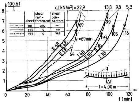
same fire resistance. Obviously the composite action - well known to be highly beneficial for the ultimate load under ambient temperature - has no significant improving effect for the load bearing under fire conditions. Thinking of the heating behavior explained before, this result does not surprise:
