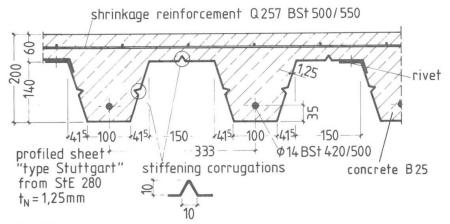
Fig. 8 Sheet-supported reinforced concrete slab in demo-building
