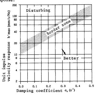
Figure 3. Illustration of impulse velocity response (left) and diagram for rating of floor impulse response (right).
