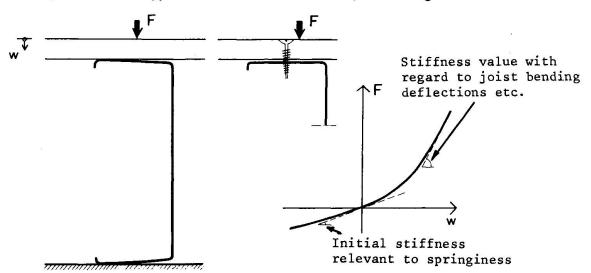
Figure 4. Illustration of low initial rigidity due to flange plate bending or bad function of self-tapping screws. F = force, w = deflection.
