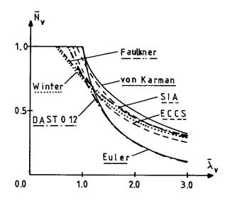
Figure 3: Several proposals for plate buckling curves.
