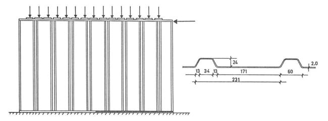
Fig. 3 Arrangement of panel testing. Section of the panel. (Panel h = 1270 mm, l = 1995 mm.)
