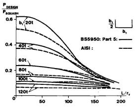
Fig. 15. Failure loads for plain channel columns
