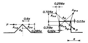
Fig.9 Shear centers of distortion
