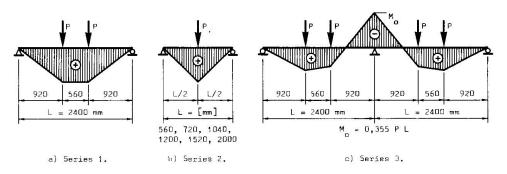
$\underline{\text{Fig. 2}}$  : Static system for the tests.
