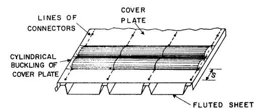
Fig. 1 - Cellular Panel with Flat Cover Plate
