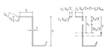
Fig. 3 Calculation of the effective crosssection for a Z-and C-profile.
