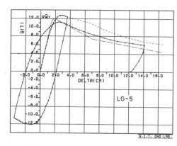
Fig.4 Load-Deflection Curve of LG-5
