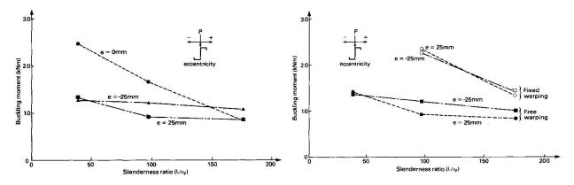
Fig. 6 Variation of buckling load with slenderness ratio and horizontal eccentricity.
