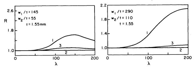
Fig. 3 Interaction of local and overall buckling - tubes  $(F_y/E = .0017)$
