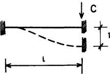
Fig. 3 Model for the spring stiffness
