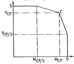
Fig. 5 Moment/shear interaction diagram
