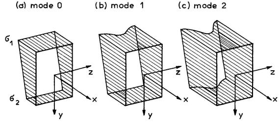
Fig. 3 Modes of the cross-section behaviour
