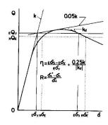
Fig.9 Evaluating Method of Deformation Capacity
