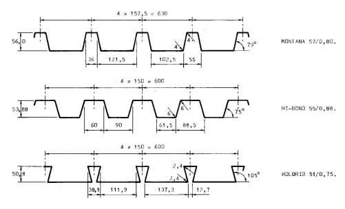
Fig. 1 : Profiled sheeting sections.
