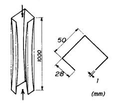
Fig.13 Distortional buckling
