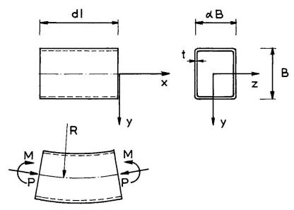
Fig. 1 Compression and bending of a segment
