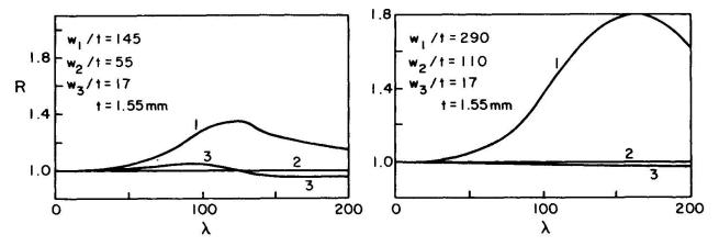
Fig. 2 Interaction of local and overall buckling - C sections  $(F_y/E = .0017)$
