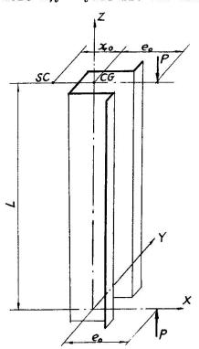
Fig. 1 Singly symmetric open section under eccentric load
