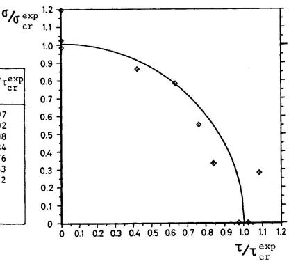
Fig. 6 Buckling stresses at combined axial load and shear load.
