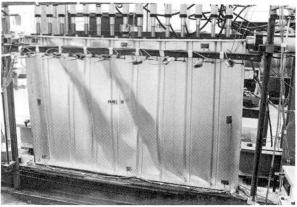
Fig. 5 Buckling pattern after testing. Panel P9 and P10 resp.
