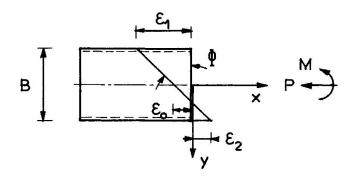
Fig. 2 Strain distribution of a section
