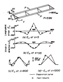
Fig.12 Distortion of a bar with bulkheads
