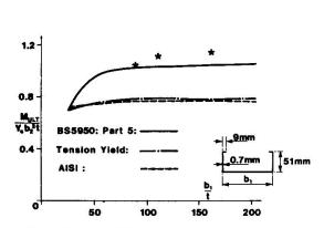
Fig.13. Failure moments for channels with small lips
