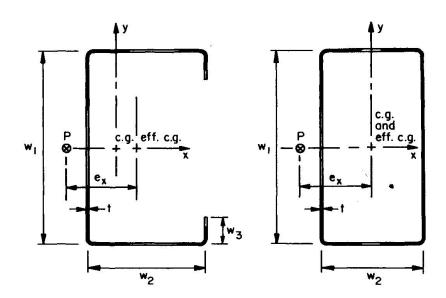
Fig. 1 Section geometry and generalized effective section
