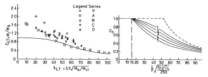
Fig. 3 Lateral-torsional buckling of beams containing slender plate elements
