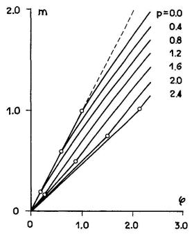
Fig. 4 Moment-curvature-thrust relationships
