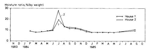
Fig. 11 Example of results. Moisture is measured by means of built-in wooden rounds placed between the concrete slab and the cellular plastic insulation. The large increase in the moisture ratio in June-July was caused by the leaks in connection with raising the steel construction. Apart from this incident the moisture ratio has remained during the whole period at an even and low level (8-10%). The moisture ratio values refer to the moisture ratio in the moisture measuring gauges.
