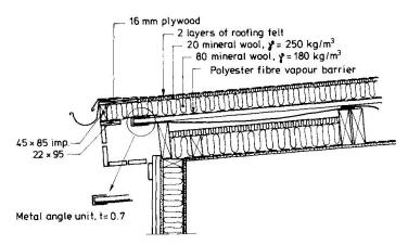
Fig. 4 Rebuilt roof. The ventilation was closed off. As the joints in the metal sheeting were not tight, a sheet of roofing felt was laid on the metal as a vapour barrier. The additional insulation was nailed on.
