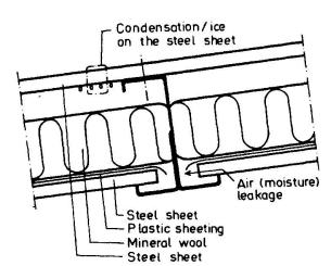
Fig. 5 A very poor design leading to condensation problems
