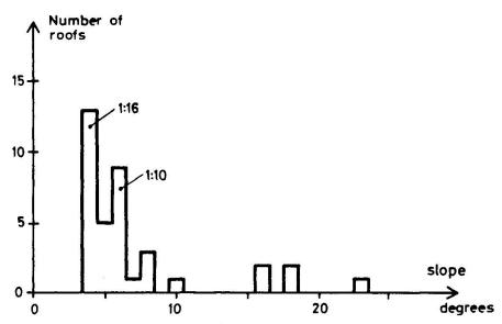
Fig. 7 Roof slopes for investigated roofs
