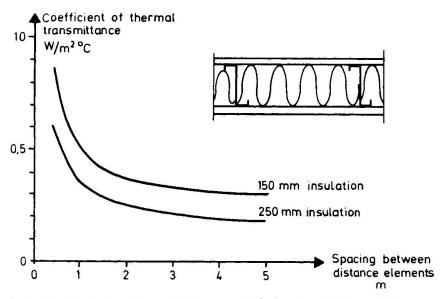
Fig. 3 Calculated value of the coefficient of thermal transmittance U.
