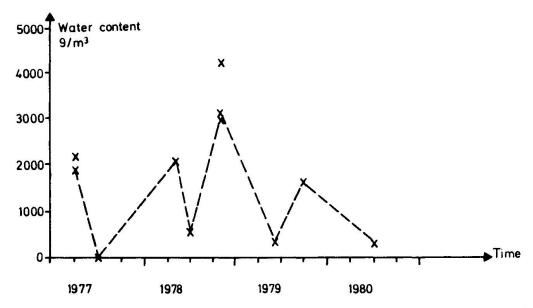
Fig. 9 In situ tests. Measured variation of moisture content for a double steel sheet roof. The moisture disappears during the summer period.
