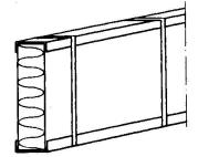
Fig. 2 Different types of spacer elements, especially designed to minimize heat loss.
