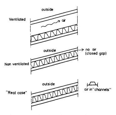
Fig. 4 Different design principles for insulated roofs
