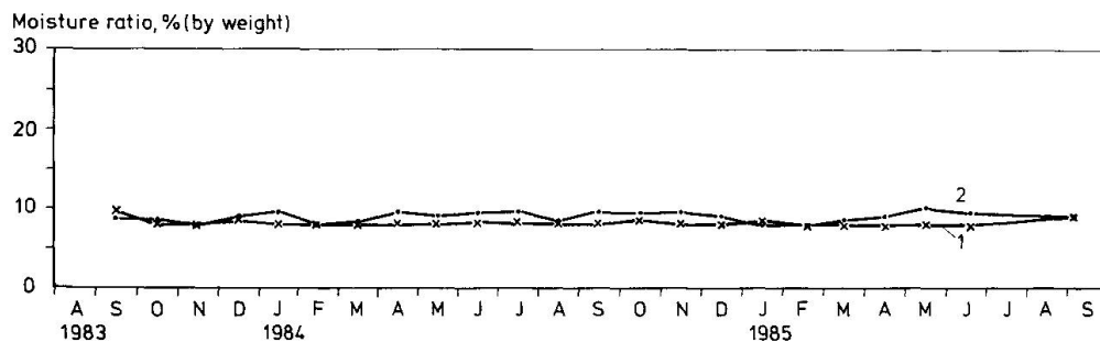
Fig. 8 Example of results. Moisture and temperature are measured both in the air space, line 1 and immediately below the new weatherproof layer, line 2. Since additionally insulating the roof the moisture ratio in the roof has remained for the whole period at a low level, c. 8% in the air space and c. 10% under the new weatherproofing. However, the moisture ratio at one of the measurement points immediately below the new weatherproofing was c. 20%, which indicates that moisture has been enclosed. Moisture is measured by means of built-in moisture-measure gauges; figures refer to the moisture ratio in these rounds.
