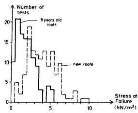
Fig. 4 Measured strength of roofs with glass wool and mineral wool - comparison between old and new strength,
