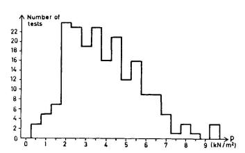
Fig.3 Measured strength of roofs with glass wool and mineral wool
