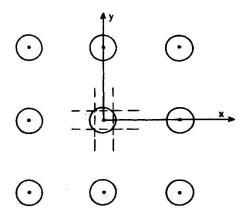
Fig. 7 Mechanical fasteners. Possible folding lines for the washers are indicated.
