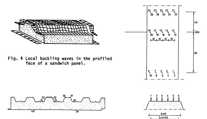
Fig. 5 The location of strain gauges and inductive displacement transducers for measuring the global and local deformations.
