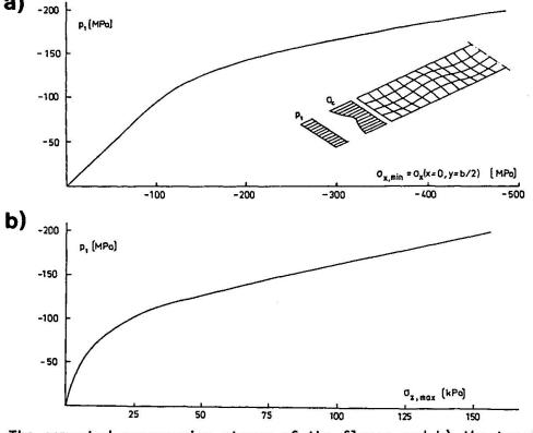
Fig.8 a) The computed compressive stress of the flange and b) the tensile stress of the joint of the tested sandwich panel using the method presented by Linke /3/. The initial deflection is  $w_0$  = 0.1 • t.
