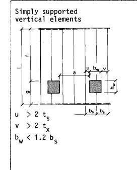
Bending moments and shear forces according to the following formulae shall be less than allowable values for the actual sandwich panel:
