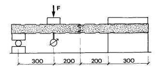
Fig. 7 Testing of the joints between sandwich elements
