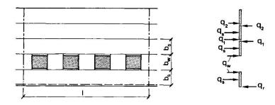
Fig. 9 Windows in horizontal elements
