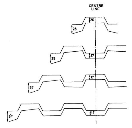
Mid-span deformation for 3m span samples carrying  $2 \text{ kN/m}^2$ . Fig. 3
