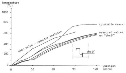
$\underline{\text{Fig 10}}$  An example of the theoretical and test temperatures in the composite slab
