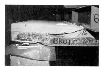
Fig 3 Panel deformation at ultimate load
