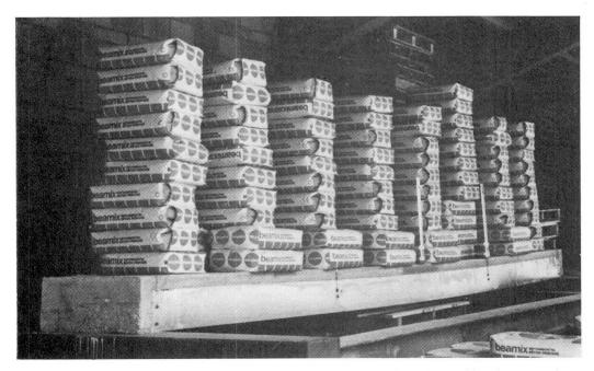
Fig. 11 Composite deck element under test loading (field test)
