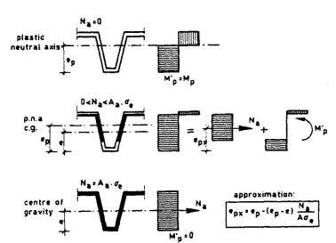
$\underline{\text{Fig. 9}}$  Position of the tensile stress resultant N<sub>a</sub> for various values of M.
