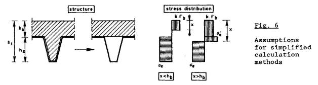
There are two possible cases to be considered, depending on the hight x of the compression stress block. For the type of floors under consideration practically ever is  $x > h_b$ . Although much simplified now, the calculation for this case is still elaborate. Therefore, a further simplification is introduced.
