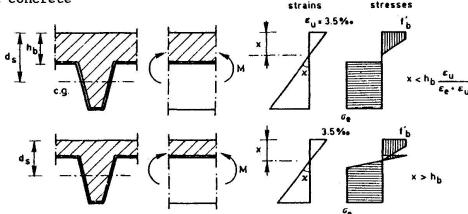
Fig. 2 Strain- and stress distributions
