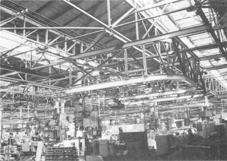
Fig. 3 roof trusses with hanging-crane
