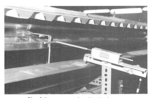
Fig. 2 Measurements of purlin displacements
