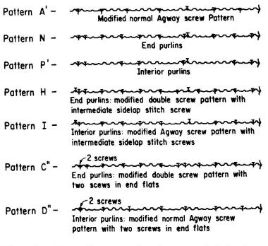
Fig. 5 - Screw Patterns for Recommended Designs
