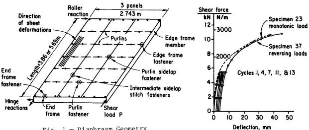
Fig. 1 - Diaphragm Geometry and Connector Geometry
