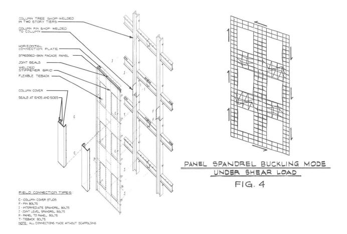
FIG.3 ONE MELLON BANK CENTER STRESSED SKIN TUBE INTERFACE
