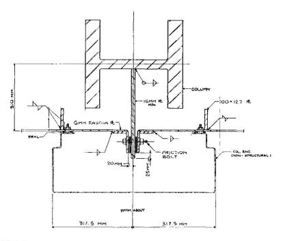
FIG.8 PANELS-TO-COLUMN VERTICAL CONNECTION
