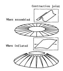
Fig. 1. System of stainless steel membrane roof
