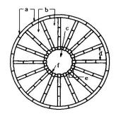
Fig. 2. Members of stainless steel membrane roof
