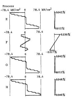
Distribution of Distribution of stress intensity strain at fixed at fixed end end
