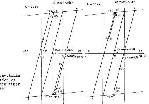
Fig. 15. Stress-strain relation of surface fiber stress
