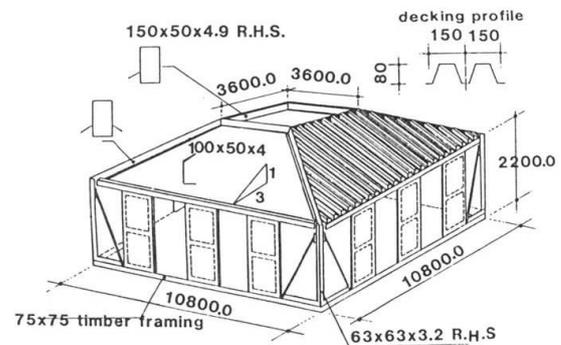
Fig. 1 MACE Type 30 unit as tested.
