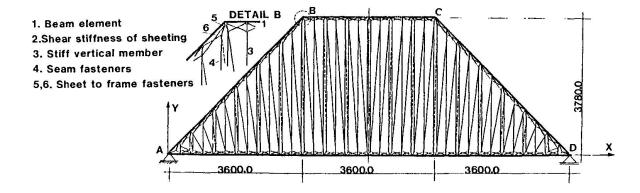
Fig. 8 Full truss simulation of MACE panel
