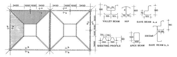
Fig. 4 Plan of tested Pyradome structure
