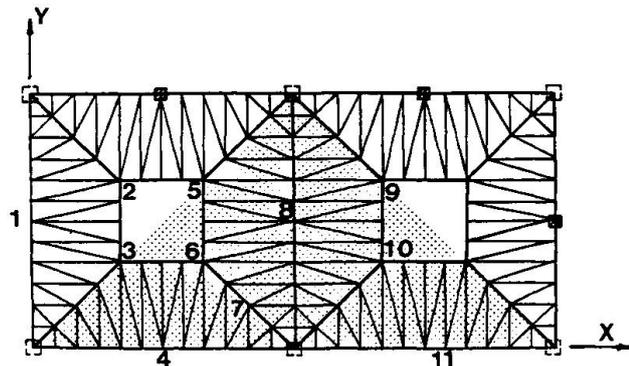
Fig. 13 Plan of model for analysis of Pyradome.
