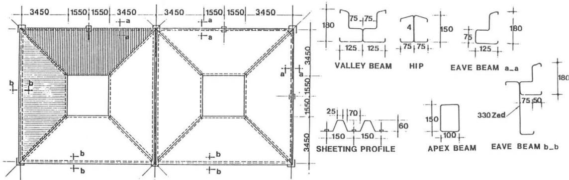
Fig. 4 Plan of tested Pyradome structure
