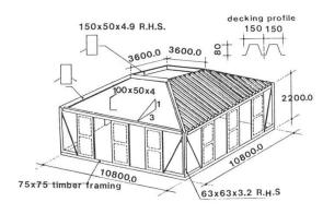
Fig. 1 MACE Type 30 unit as tested.
