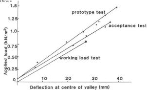
Fig. 6 Typical load-deflection curves for Pyradome.
