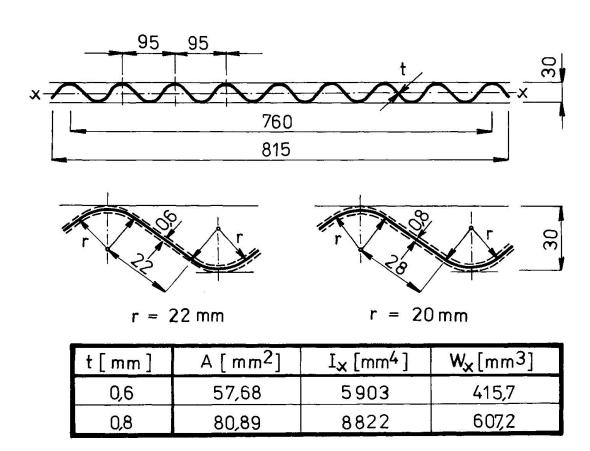
Fig. 1 Cross section and characteristics of the specimens
