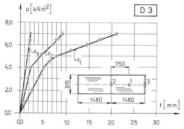
Fig. 4 Load - Deflection Relationship for Two-span Panel
