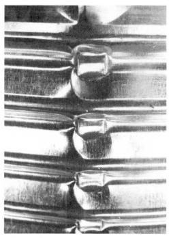
Fig. 6 Support Crippling
