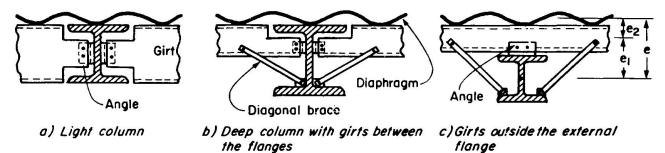
Fig. 1 — Girt-to-column connections.
