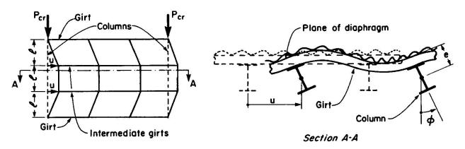
Fig. 5 — Flexural-torsional buckling mode.
