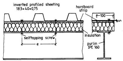
Fig. 2 Roof-construction with thermal insulation
