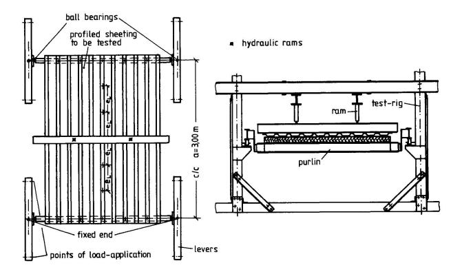
Fig. 3 Test Configuration
