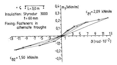
Fig. 4 Example of the graphical evaluation
