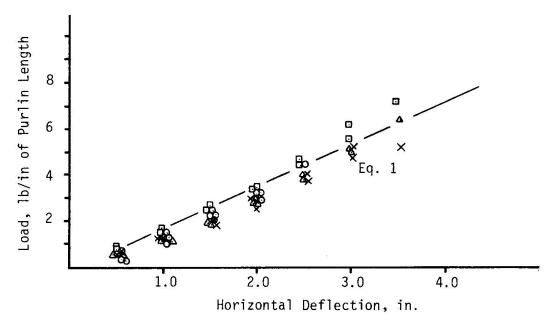
Fig. 9 - "F" for Typical Roof Systems Having .061" Purlin
