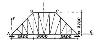
Fig. 9 Simple truss simulation
