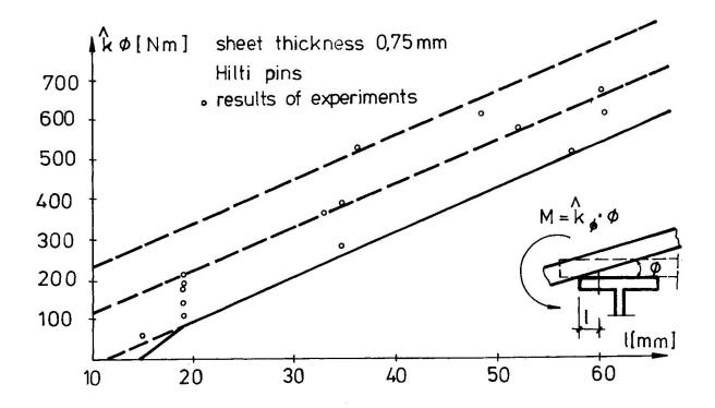
Fig.1. The rotational rigidity of a flange to corrugated sheet attachement.
