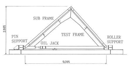
Fig.8 Test Set-up of Frame
