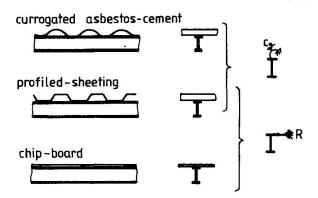
Fig. 1 Stabilizing by adjacent components
