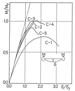
Fig.4 Load-Deflection Curves of Channel Steel
