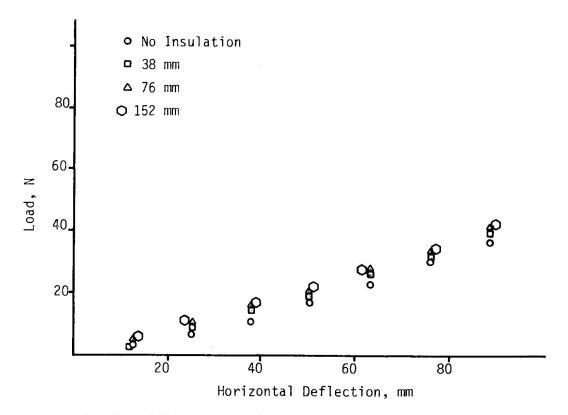
Fig. 6 - Affect of Insulation Thickness
