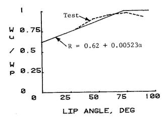
Fig. 3 Strength Ratio versus Lip Angle
