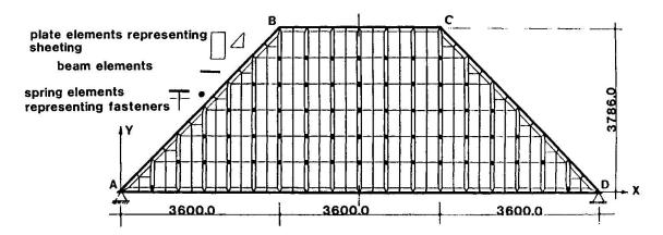
Fig. 7 Finite element model of MACE roof panel.
