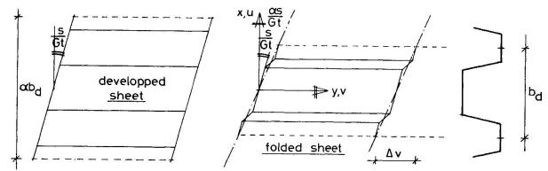
Figure 2: shift and warping due to shear strain
