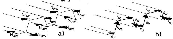
Figure 6: a) internal longitudinal forces concentrated in the foldlines
