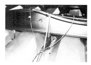
$\underline{\text{Fig.5}}$  Local Buckling of Channel Steel
