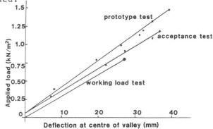
Fig. 6 Typical load-deflection curves for Pyradome.
