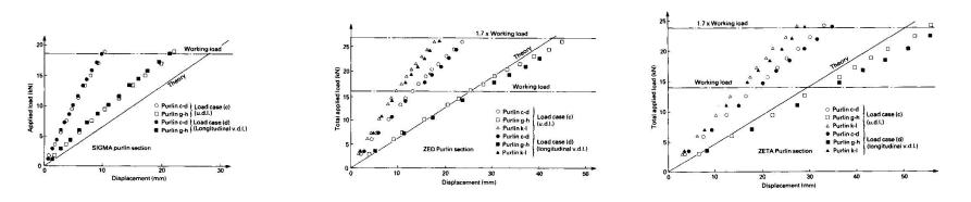
Fig. 4 Load displacements for u.d.l and longitudinal v.d.l
