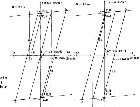
Fig. 15. Stress-strain relation of surface fiber stress
