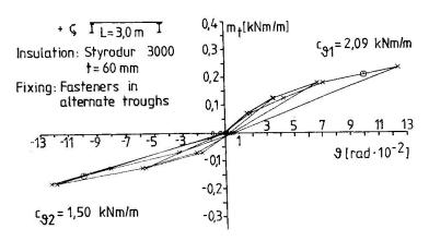
Fig. 4 Example of the graphical evaluation
