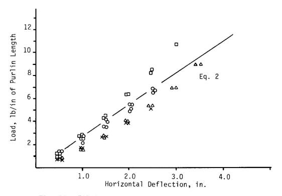
Fig. 10 - "F" for Typical Roof Systems Having .120" Purlin
