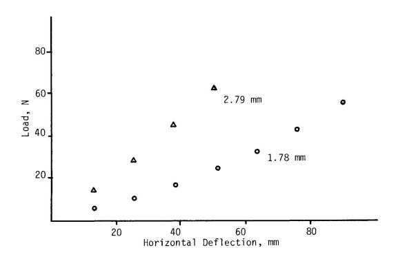
Fig. 2 - Affect of Purlin Thickness
