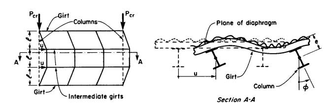
Fig. 5 — Flexural-torsional buckling mode.
