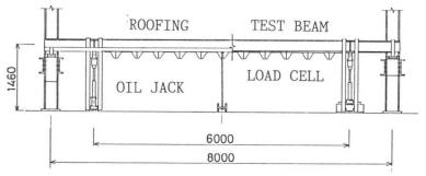
Fig.3 Test Set-up of Channel Steel
