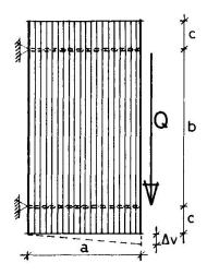
Figure 8: diaphragm with overhang
