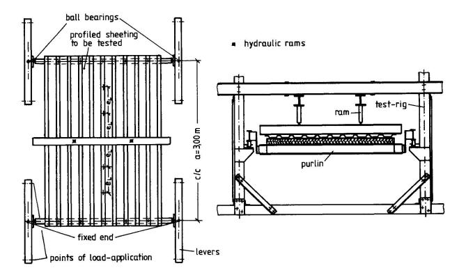
Fig. 3 Test Configuration
