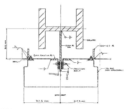
FIG.8 PANELS-TO-COLUMN VERTICAL CONNECTION
