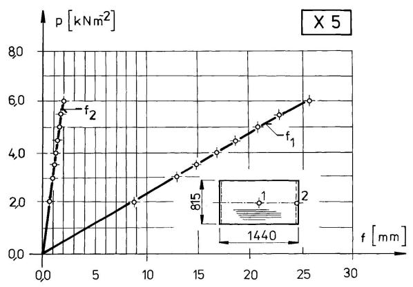
Fig. 3 Load - Deflection Relationship for Single-span Fanel between the outside atmospheric pressure and inside the test frame. The test setup and instrumentation are shown in Fig. 2. The support settlements and maximum span deflections were measured using a stroke dial gages.
