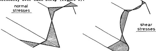
Figure 5: membrane stresses due to warping
