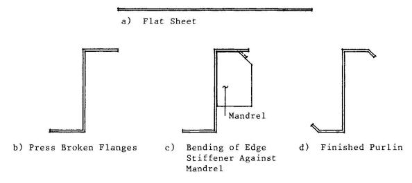
Fig. 1 Z-Purlin Fabrication Procedure
