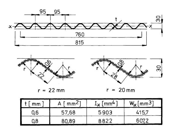
Fig. 1 Cross section and characteristics of the specimens
