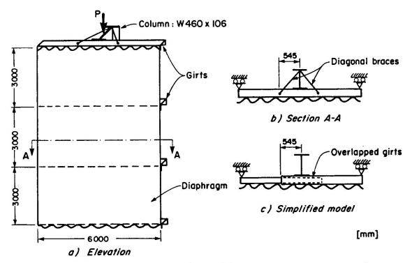
Fig. 6 — C.G.D. sub-system with diagonal braces (pin -ended column)
