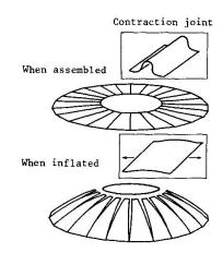
Fig. 1. System of stainless steel membrane roof
