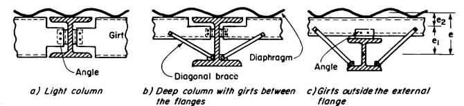
Fig. 1 — Girt-to-column connections.
