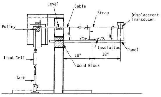
Fig. 1 - Test Apparatus
