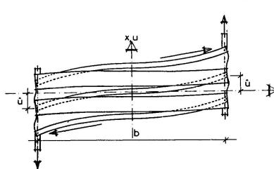
This is shear deformation of a diaphragm due to distortion. The latter in combination with the previous result of 2.1 yields the complete kinematic condition for profiled sheeting in shear:
