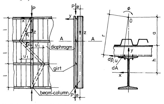
Fig. 2, A beam-column and its bracing
