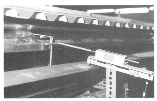
Fig. 2 Measurements of purlin displacements
