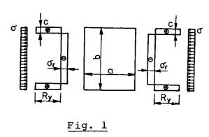
When the web has been cooled, the longitudinal stresses near the weld remain close to the yield stress and are balanced by compressive stresses. It is advantageous /for the sake of calculations/ to work with idealized residual stresses, which very satisfactorily describe the actual stress distribution. A simple rectangular tension distribution of the residual stresses would be suitable for using in the analysis /Fig. 1/.
