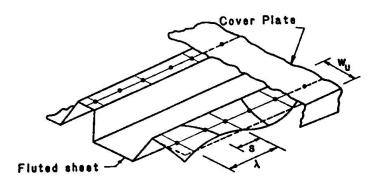
Fig. 5. - Buckling of Outstanding Unstiffened Flanges
