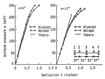
Fig. 3 - P- $\delta$  Curves for Two-Span Continuous Panels
