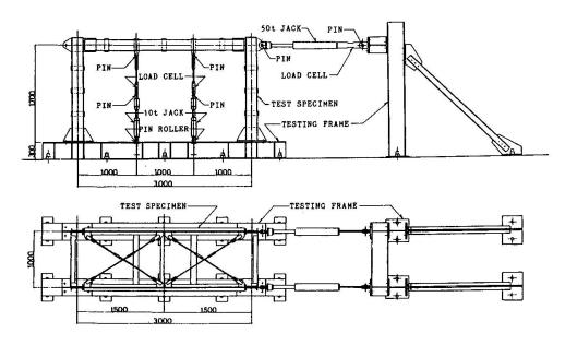
Fig.1 Set-Up of Frame Test
