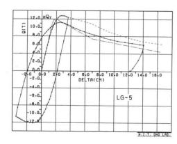
Fig.4 Load-Deflection Curve of LG-5
