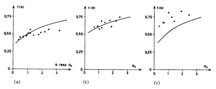
Fig. 8 Measured  $\delta_{\rm m}/\Sigma\delta$  (left),  $\epsilon_{\rm m}/\Sigma\epsilon$  in midspan (middle) and  $\epsilon_{\rm m}/\Sigma\epsilon$  for support moment. The curves are theoretically calculated.
