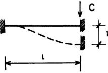
Fig. 3 Model for the spring stiffness
