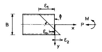
Fig. 2 Strain distribution of a section
