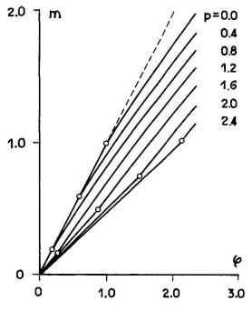
Fig. 4 Moment-curvature-thrust relationships
