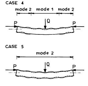
Fig. 6 An eccentrically loaded beam-column (possible cases)
