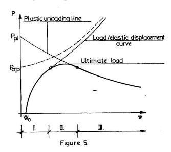
Assuming that the transformation should take place at an identical value of inplane displacement (and using the legend applied in Figure 6), we can determine the following relation between the characteristic values of out-of-displacement:
