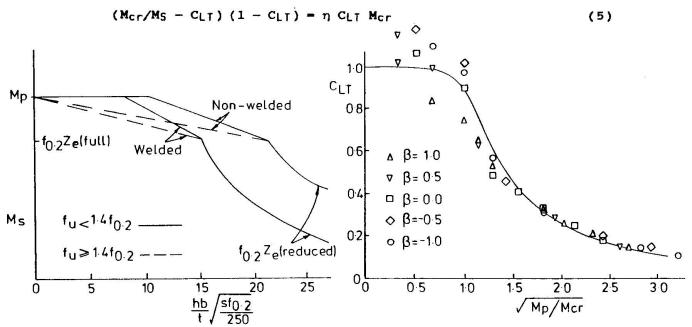
Fig. 1 Moment Capacity  $M_s$  - plotted for a beam with  $f_u$  = 1.2 $f_{0,2}$  or  $f_u$  = 1.4 $f_{0,2}$  with capacity controlled by an internal element
