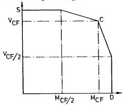
Fig. 5 Moment/shear interaction diagram
