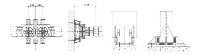
Fig. 8 - Constructional details of the seismic supports.
