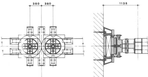
Fig. 8 - Constructional details of the seismic supports.
