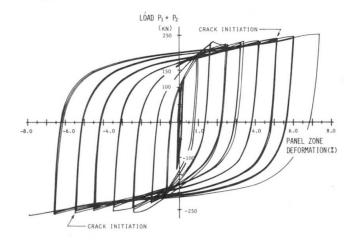
Fig. 8 Load-Deformation Curves of Joint D
