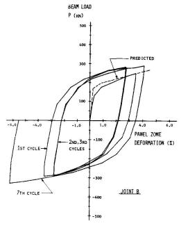
Fig. 4 Load-Deformation Curves of Joint B
