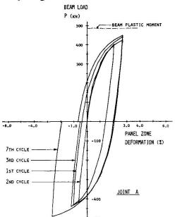
Fig. 3 Load-Deformation Curves of Joint A
