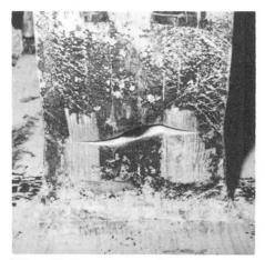
Fig. 7 Fracture of Beam Flange in Joint D
