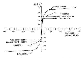
Fig. 9 Skeleton Curves of Joint D
