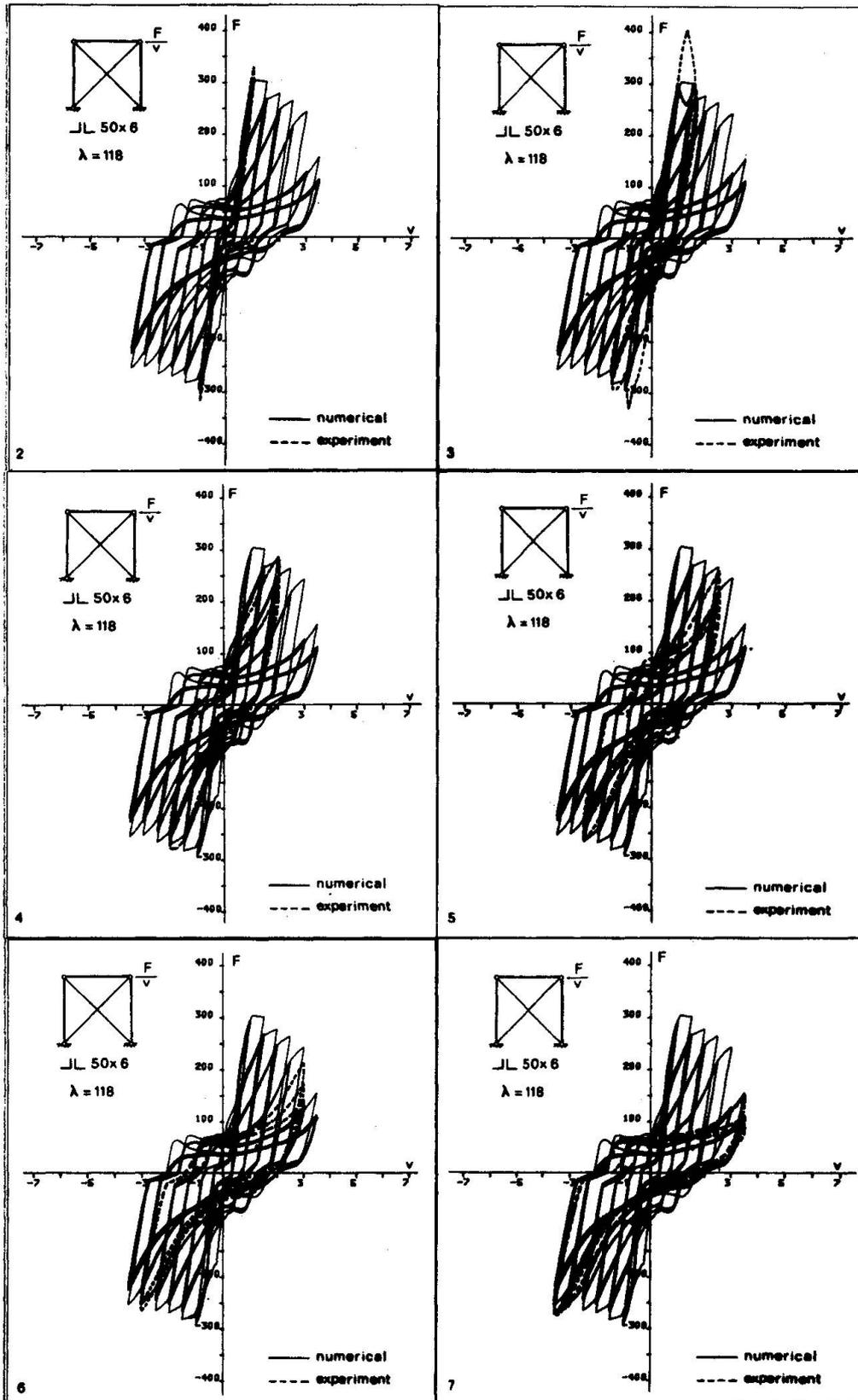
Fig. 4 - Numerical results on the bracing of Fig. 3
