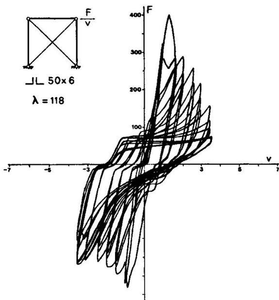
Fig. 3 Experimental test on a cross section truss bracing  $F$  (KN) -  $v$  (cm)
