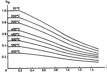
Fig. 8 Relationship between non-dimensional buckling load  $\bar{N}_{\theta}$  and slenderness factor  $\bar{\lambda}$  at varying steel temperature  $T_g$  for unrestrained axially loaded steel columns [23]
