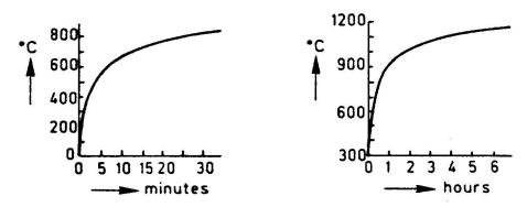
Fig. 2 Standard temperature-time curve [3]
