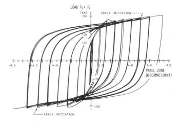
Fig. 8 Load-Deformation Curves of Joint D
