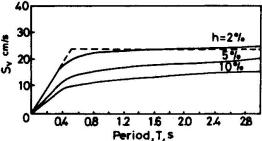
FIG.2 Average velocity response spectrum
