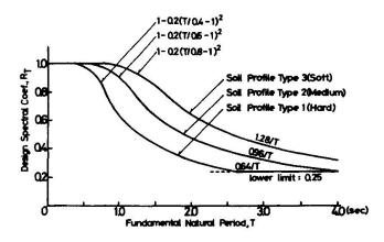
FIG.1 Design spectral coefficient, R,
