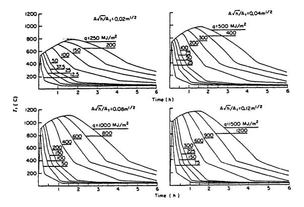
Fig. 3 Gas-temperature-time curves for a complete, fully developed compartment fire with varying values for the fire load density q and the opening factor  $A/h/A_{+}$  according to Pettersson, Magnusson and Thor [4]
