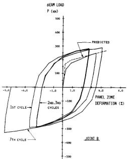
Fig. 4 Load-Deformation Curves of Joint B
