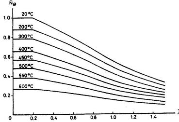
Fig. 8 Relationship between non-dimensional buckling load  $\bar{N}_{\theta}$  and slenderness factor  $\bar{\lambda}$  at varying steel temperature  $T_g$  for unrestrained axially loaded steel columns [23]
