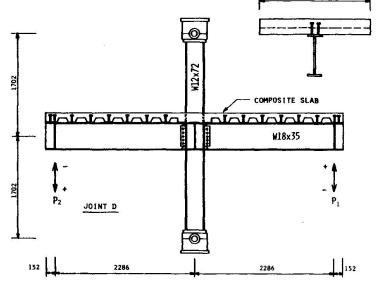
Fig. 2 Dimensions and Details of Joint D
