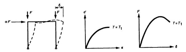
Fig. 9 Structural design at elevated temperatures with an incremental elastoplastic analysis
