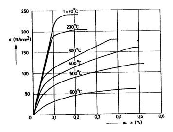
Fig. 5 Stress-strain relationships for Fe 360 at elevated temperatures
