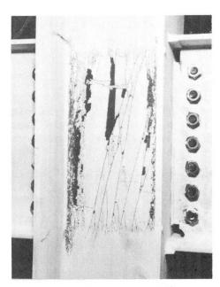
Fig. 5 Panel Zone Yielding of Joint C
