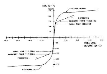
Fig. 9 Skeleton Curves of Joint D
