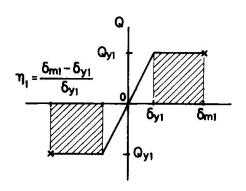
FIG.3 Cumulative ductility ratio
