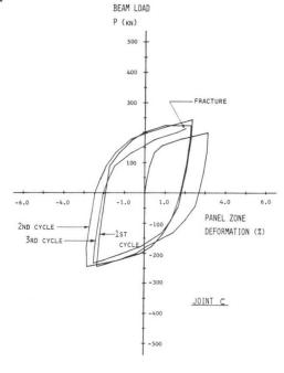
$\frac{\text{Fig. 6}}{\text{of Joint C}} \text{ Load-Deformation Curves}$
