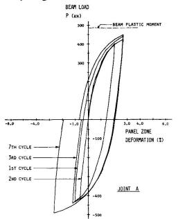
Fig. 3 Load-Deformation Curves of Joint A
