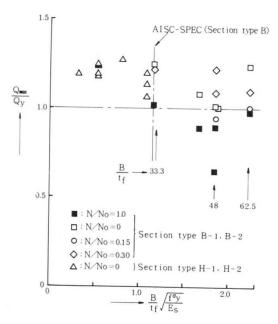
Fig.7 Maximum load and B/t<sub>f</sub>
