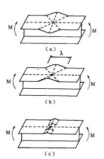
Fig.3 Buckling mode of steel
