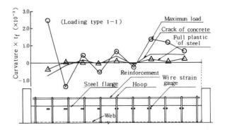
Fig.5 Deformation of steel flange (Pw=0.2%)
