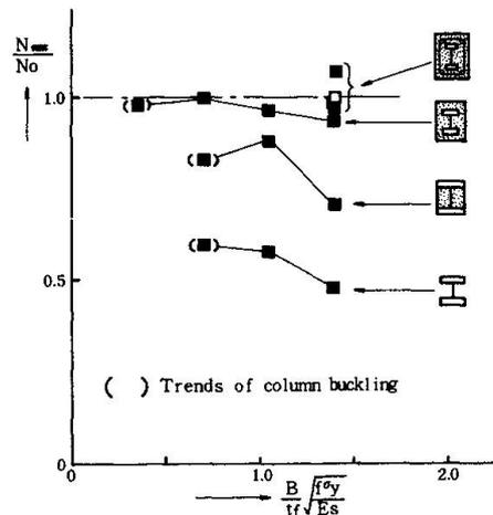
Fig.8 Maximum load and  $B/t_f$  (Loading type 1-1)
