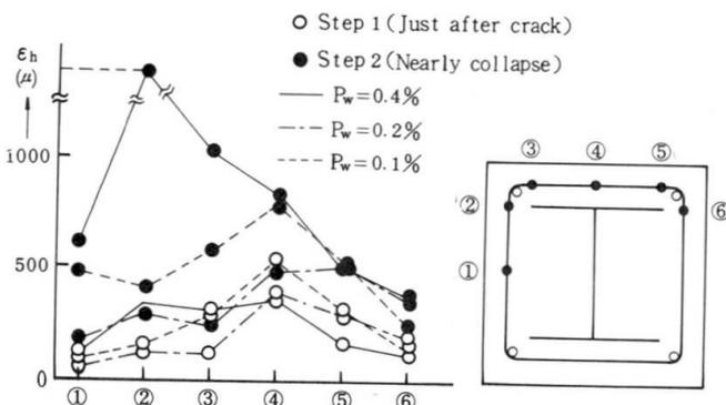
Fig.6 Strain of hoop reinforcement
