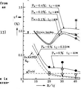
Fig.17 Limit strain of steel flange (Loading type 1-1, section type H-1, H-3, H-4)
