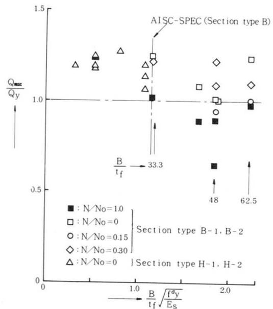
Fig.7 Maximum load and  $B/t_f$  (Loading type 3, 4-1)
