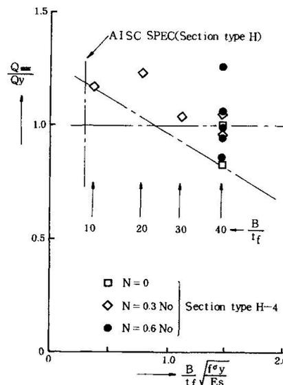
Fig.9 Maximum load and  $B/t_f$  (Loading type 4-2)
