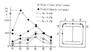
Fig.6 Strain of hoop reinforcement
