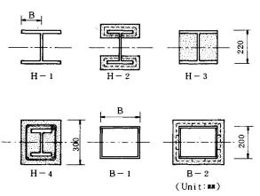
Fig.1 Section types of specimen
