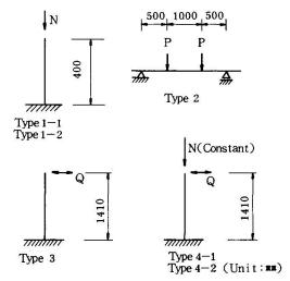
1-1, 4-1 Steel is only compressed 1-2, 4-2 Steel and concrete are compressed
