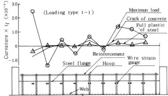
Fig.5 Deformation of steel flange ( $P_w=0.2\%$ )
