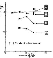
$\frac{\text{Fig.8}}{\text{(Loading type 1-1)}} \frac{\text{Maximum load and B/t}_f}{\text{(Loading type 1-1)}}$
