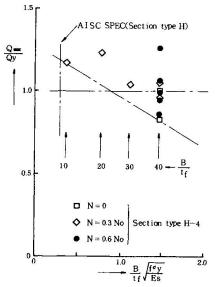
$\frac{\text{Fig.9}}{\text{(Loading type 4-2)}} \frac{\text{Maximum load and B/t}_f}{\text{(Loading type 4-2)}}$
