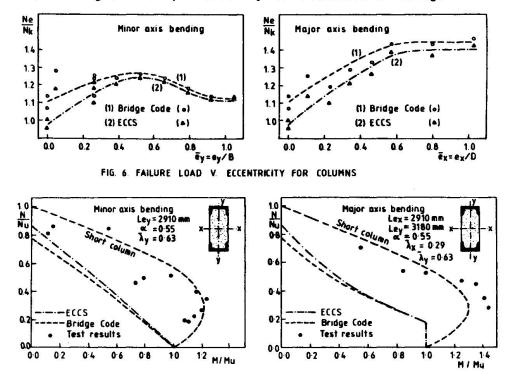
FIG. 7. INTRACTION CURVES UNDER UNIAXIAL BENDING FOR COLUMNS USING 152 x 76 STEEL CHANNELS
