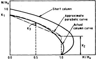
FIG. 1. TYPICAL INTRACTION GRAPHS FOR COMPOSITE COLUMNS.
