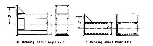
FIG: 3. DETAILS OF COLUMN ENDS SUBJECTED TO LARGE ECCENTRICITIES
