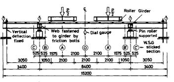
Fig.13 Ordinary span test in continuous beam
