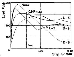
Fig.3 Typical load-slip curves
