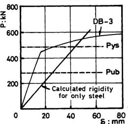
Fig.16 Load-deflection curves of DB-3
