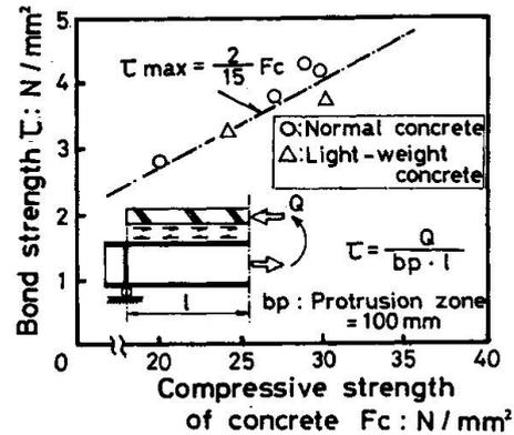
Fig.11 Relation between concrete strength and bond strength
