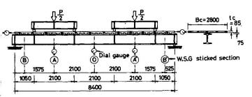
Fig. 12 Ordinary span test in simple beam
