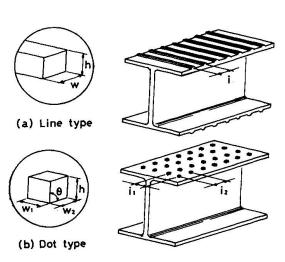
Fig.1 Type of protrusions of push-out test
