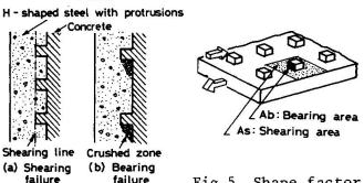
Fig.4 Failure modes
