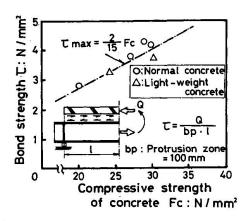
Fig.11 Relation between concrete strength and bond strength
