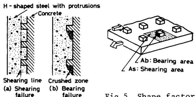
Fig.4 Failure modes
