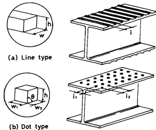
Fig.1 Type of protrusions of push-out test
