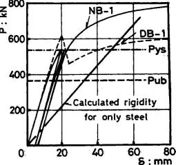
Fig.14 Load-deflection curves of DB-1 and NB-1
