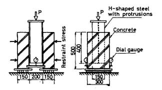
Fig.2 Test procedure of push-out test
