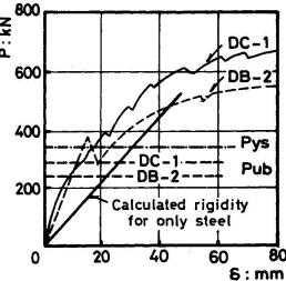
Fig.15 Load-deflection curves of DB-2 and DC-1
