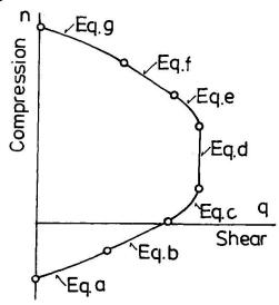
Fig.4 Schematic example of the nondimensionalied axial and shear interaction curves for the reinforced concrete portion
