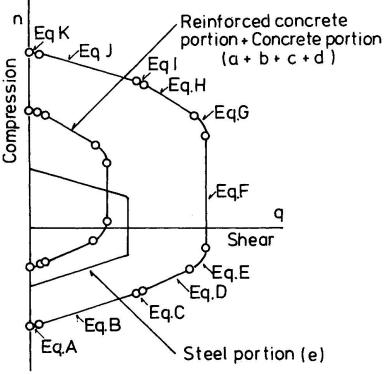
Fig.5 Schematic example of nondimensionalized axial and shear interaction curves
