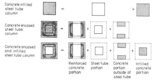
Fig.3 Physical model of stress tranfer of composite columns with steel tube
