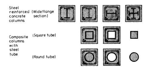
Fig.1 Classification of composite columns
