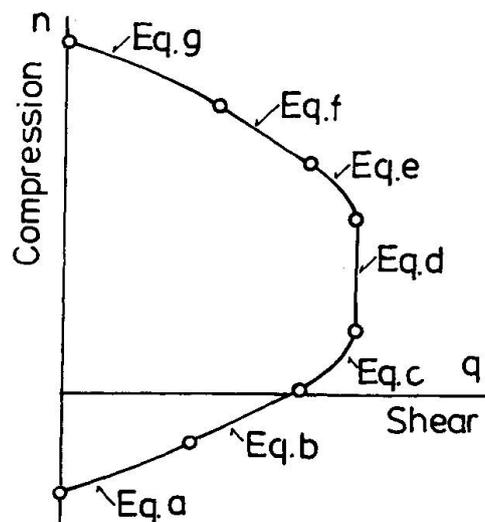
Fig.4 Schematic example of the nondimensionalized axial and shear interaction curves for the reinforced concrete portion
