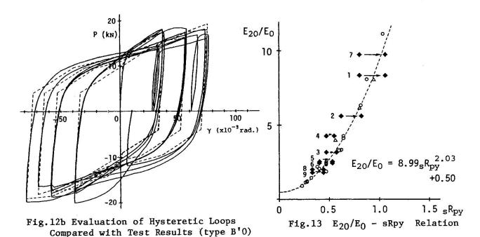
ratio of enlarged panel-zone are indicated by arrows. The energy absorption of frame subassemblage can also be evaluated by the enlargement model of panel-zone and empirical formula in figure 13.
