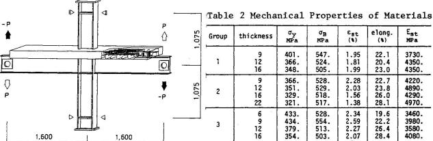
Fig.1 Configuration of Specimen
