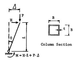
Fig. 4 Axial Force of Steel Tube
