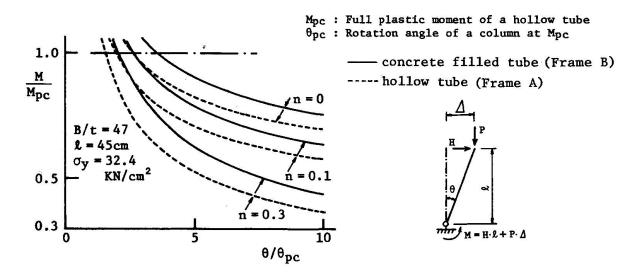
Fig. 7 Post Buckling Behavior of Columns
