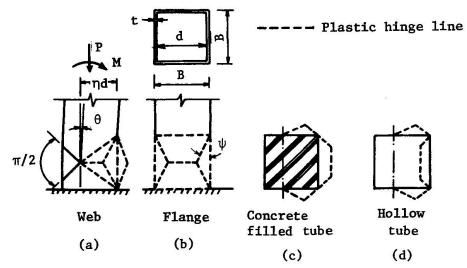
Fig. 6 Collapse Mechanism due to Local Buckling
