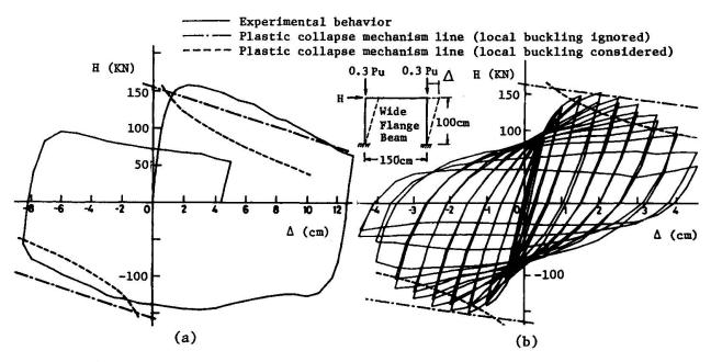
Fig. 11 Behavior of Frames Composed of Columns with B/t = 68
