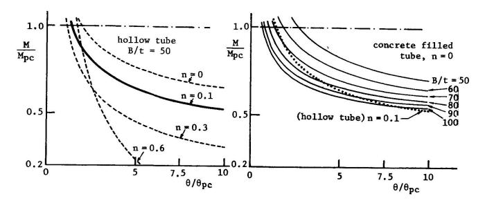
Fig. 8 Behavior of Hollow Tubes
