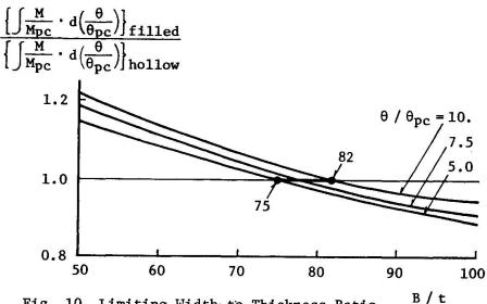
Fig. 10 Limiting Width-to-Thickness Ratio
