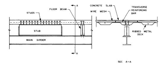
Fig. 1 Stub-Girder Floor System
