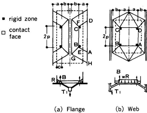
Fig. 3 Collapse Mechanism of Steel Column
