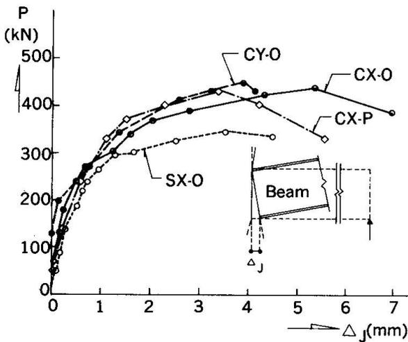
Fig. 8 P- $\Delta_j$  Relationship of Beam Flange-to-Column Connection
