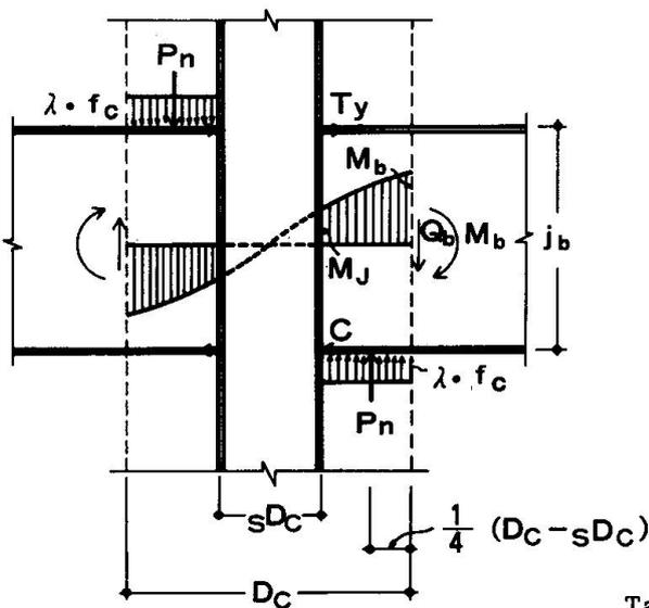
Fig. 10 Moment Resisting Model of Beam-to-Column Connections
