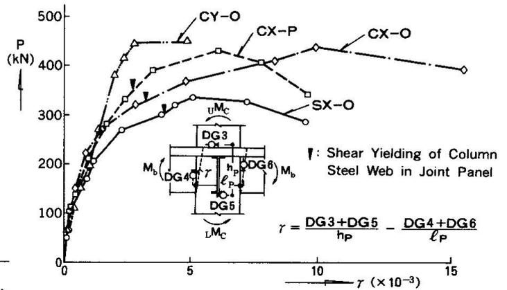
Fig. 9 P- $\gamma$  Relationship of Joint Panel
