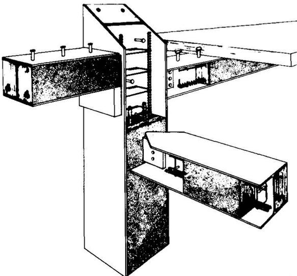
Fig. 11 Special composite cross sections
