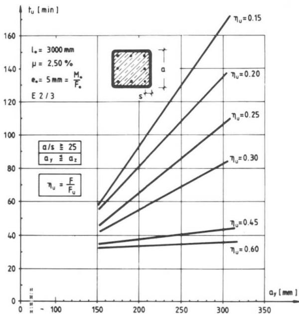
**Fig. 8** F 120-design diagram for AF columns, American wide flange shapes W 10''x 10'' to 40''x 18'' concreted between flanges ( $\beta_V/\beta_C = 355/45$  N/mm<sup>2</sup>)
