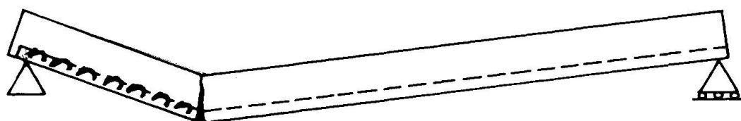
Final stage:- Mechanical bond fails and collapse occurs
