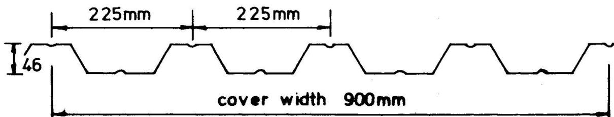
Fig.2 Precision Metal Forming CF 46.
