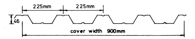
Fig. 2 Precision Metal Forming CF 46.
