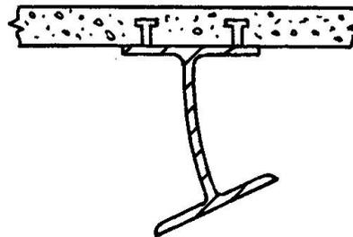
**Fig. 2** Lateral buckling
