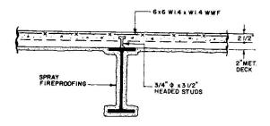
Fig.9 Typical Floor Construction Outside Core
