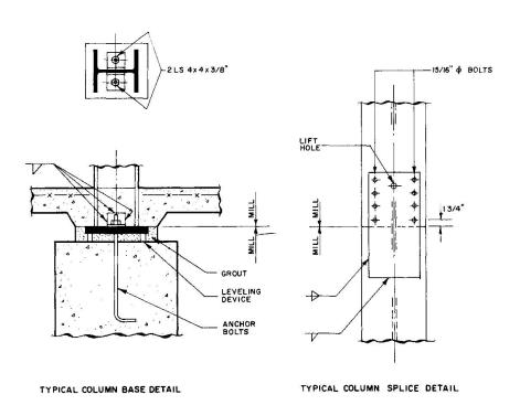
Fig.7 Typical Steel Column Details
