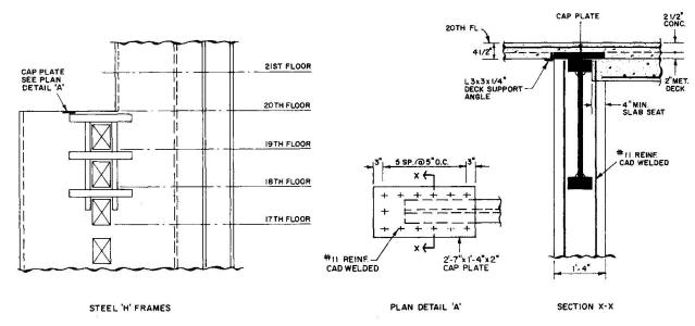
Fig.4 Structural Steel H-Frames Placed in Concrete Core
