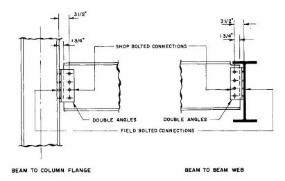
Fig.6 Typical Steel Framing Connections
