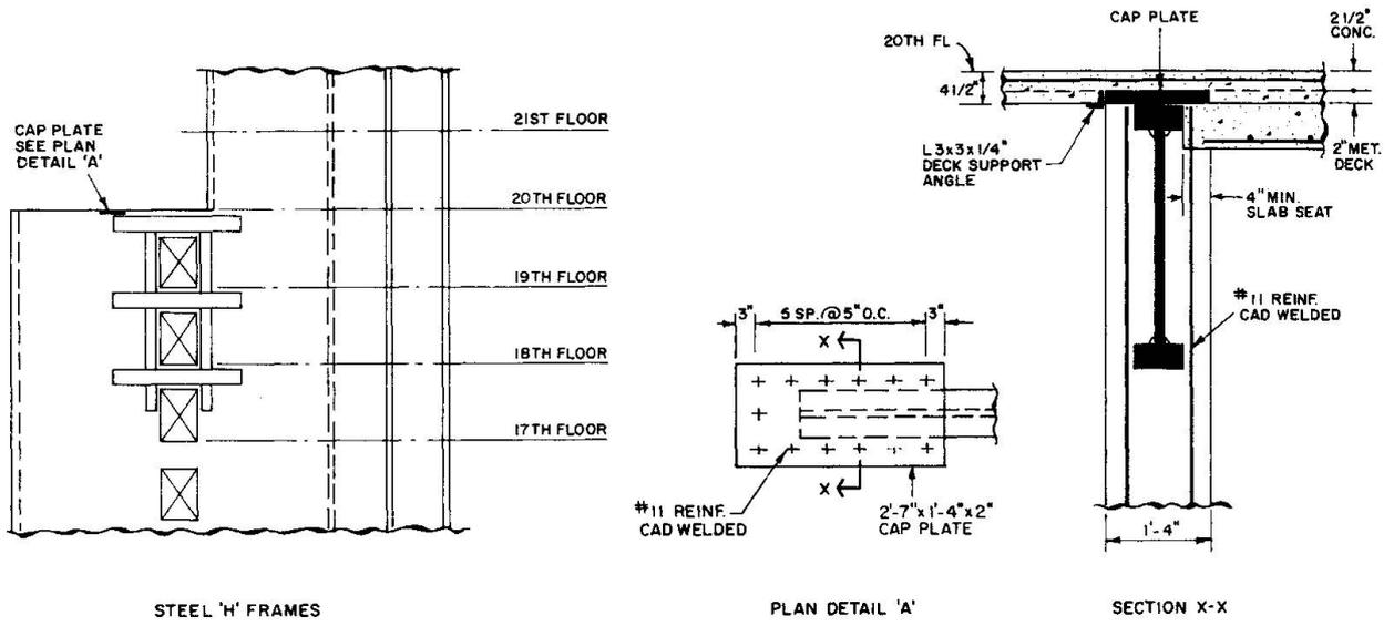
Fig.4 Structural Steel H-Frames Placed in Concrete Core
